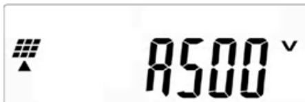
Display G: Voltage of String A
